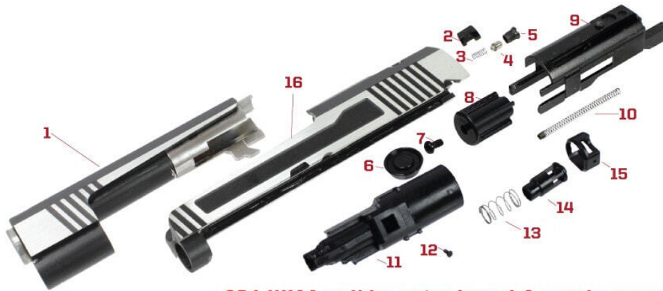
SP4-HXAA : slide, outer barrel & nozzle assembly
