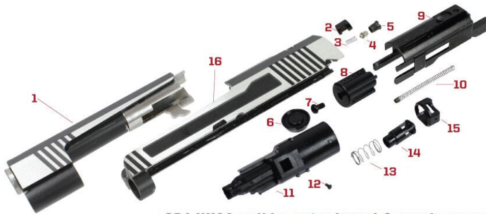
SP4-HXAA : slide, outer barrel & nozzle assembly
