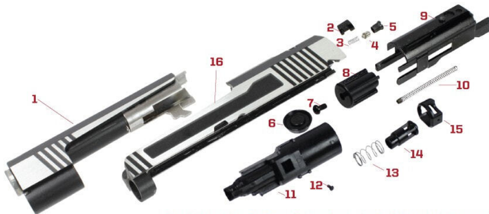
SP4-HXAA : slide, outer barrel & nozzle assembly
