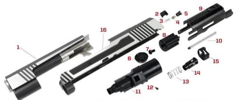
SP4-HXAA: slide, outer barrel & nozzle assembly
